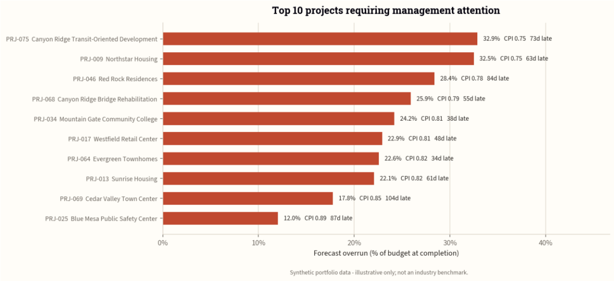
Figure 6. The ten projects carrying the largest forecast overrun, with CPI and schedule delay.
